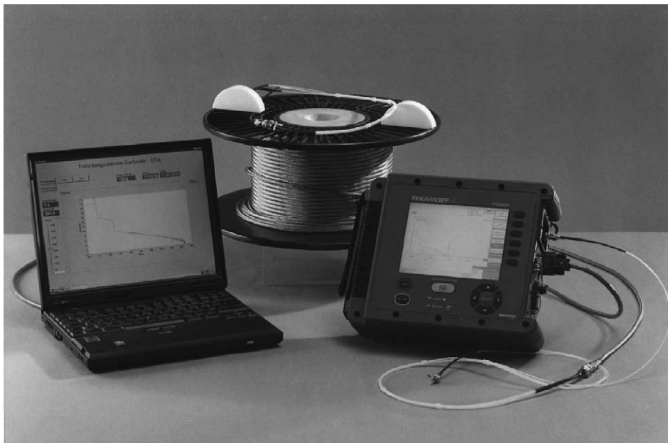
Fig. 3. Photograph of fiber-optical OTDR sensor system for continuous, spatially resolved hydrocarbon leakage control.
